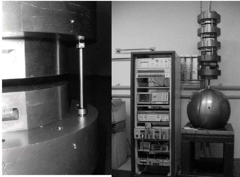
Figure 2. New vibration isolation system for the antenna.
